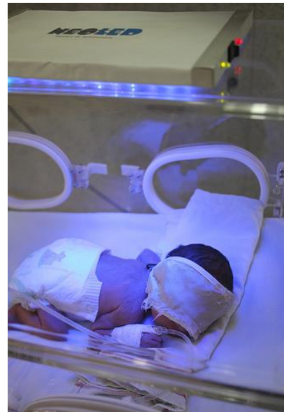
NEO Led equipment designed by Ingenimed, used for neonatal jaundice treatment. (Cusco, 2011)
